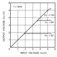
Fig. 2 VIN vs. Vout caracteristics (f = 1kHz)
